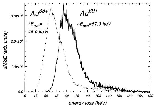
FIG. 1. Energy-loss distributions of  $\text{Au}^{33+}$  and  $\text{Au}^{69+}$  after transmission through a thin carbon foil ( $\Delta x \approx 10.4$  nm). The initial energy was  $454.4 (\pm 3)$  keV.
