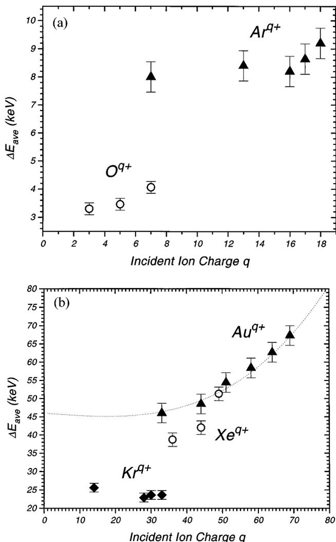
FIG. 2. Average energy loss of (a)  $\text{O}^{3,5,7+}$  and  $\text{Ar}^{7,13,16,17,18+}$ ; (b)  $\text{Kr}^{14,28,30,33+}$ ,  $\text{Xe}^{36,44,49+}$ , and  $\text{Au}^{33,44,51,58,64,69+}$  in a thin carbon foil. The dotted line is a fit to the  $\text{Au}^{q+}$  data using Eq. (1) with  $n = 1$ ,  $m = 2$  ( $\alpha = 0.0165$ ,  $\beta = 8 \times 10^{-5}$ ).
