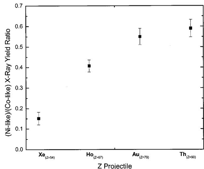
FIG. 4. Ratios of  $M$  x-ray yields for incident ions with no initial  $M$  vacancy to those for ions with one initial  $M$  vacancy as a function of the  $Z$  of the projectile for the data in Fig. 1.
