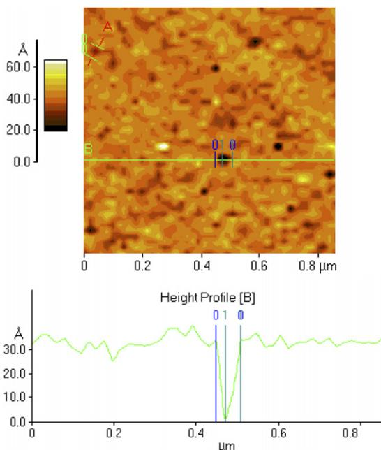
Fig. 2. AFM images of defects on the surface of a “flat” diamond type IIa surface induced by single  $\text{Xe}^{44+}$  ions.
