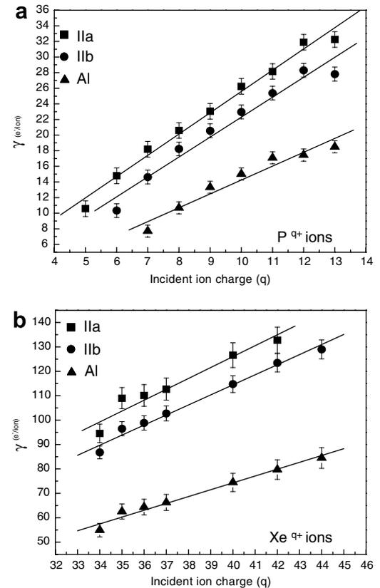
Fig. 1. Electron emission yields as a function of ion charge,  $q$ . The plots show yields for a type IIa diamond (■), a type IIb diamond (●) and an aluminium reference target (▲) for (a) phosphorous and (b) xenon ions. Solid lines are linear fits to the data.
