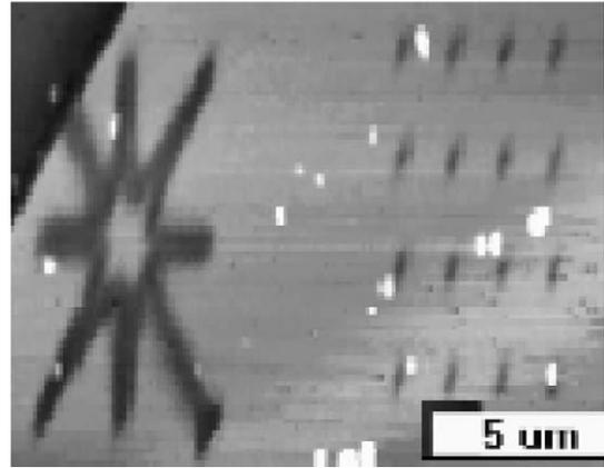
Fig. 5. Patterns formed by ion implantation with scanning probe alignment in PMMA on silicon.
