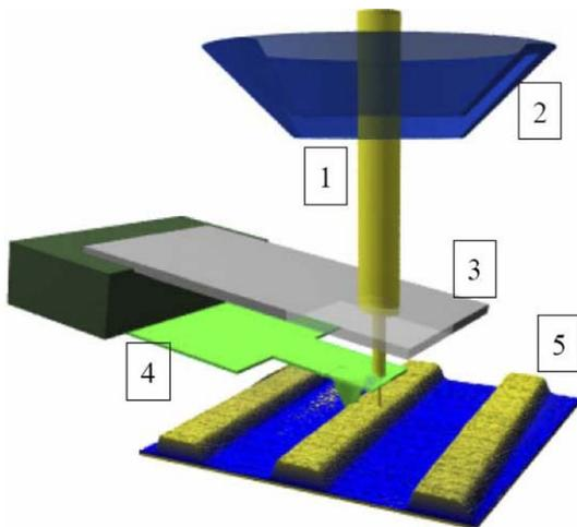
Fig. 4. Schematic of the setup for ion implantation with scanning probe alignment, showing the ion beam (1) transported through an electrostatic lens element (2) to a pre-collimating aperture (3) and the cantilever with final aperture (4). The image shows data from *in situ* imaging of 20 nm high, 1  $\mu\text{m}$  wide metal lines with 3  $\mu\text{m}$  spacing.
