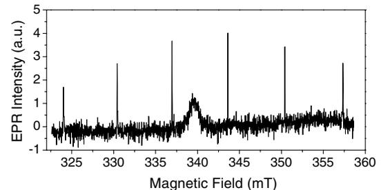
Fig. 2. x-band ESR spectrum of  $^{121}\text{Sb}$  donors in implanted  $^{28}\text{Si}$  epi layer at 5 K.
