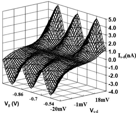
Fig. 7. Coulomb blockade ( $I_{s,d}$  vs.  $V_{s,d}$ ) and gate modulation of the source-drain current in a silicon nanowire SET with a 15 nm wire width at 4.2 K.
