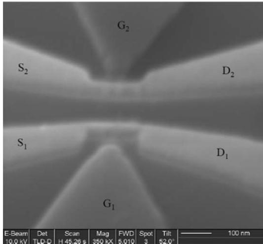
Fig. 6. Pair of single electron transistors formed in SOI.
