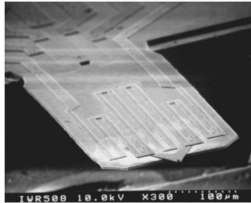
FIG. 2. Cantilever with integrated piezoresistive Wheatstone bridge, bimorph actuator, and AFM tip.
