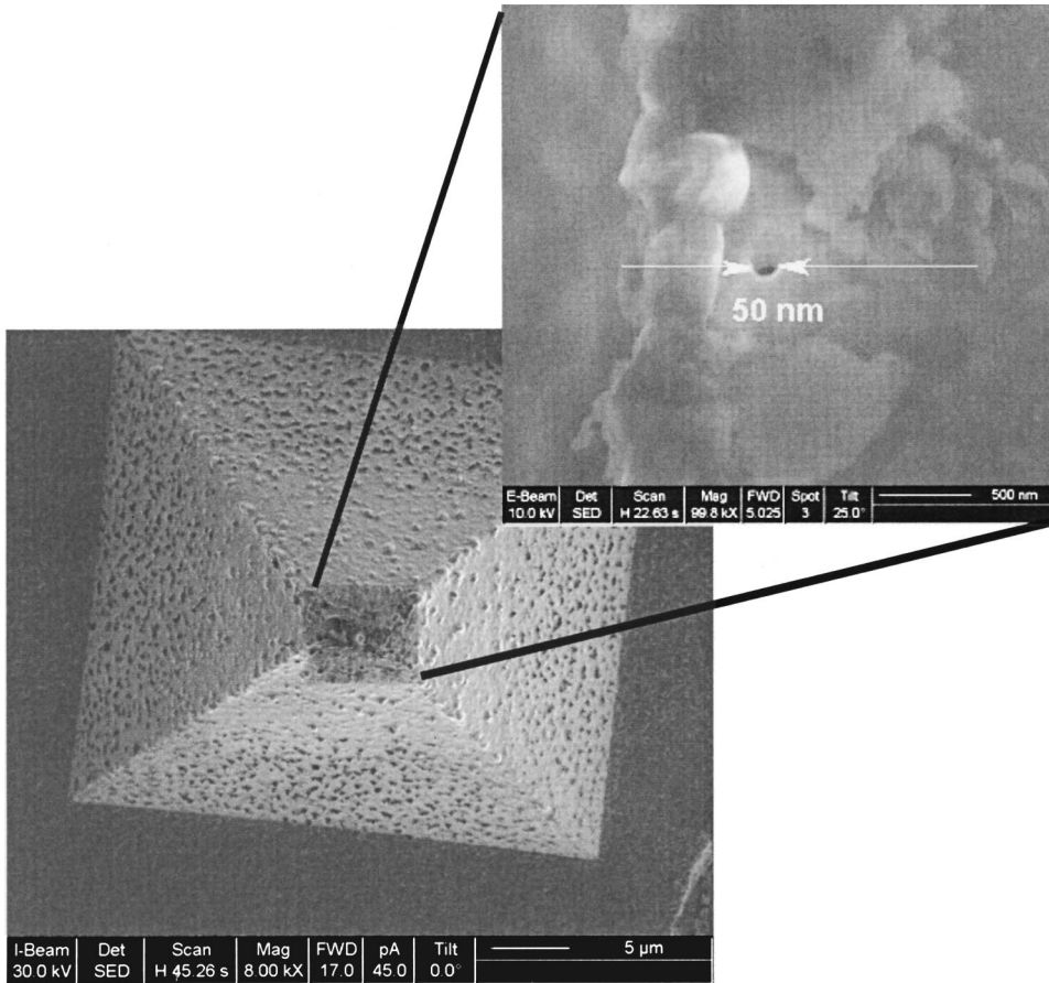
FIG. 4. SEM image of tip shape and aperture obtained by the FIB method.
