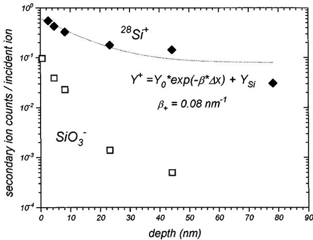
FIG. 3. SiO<sub>3</sub><sup>-</sup> (□) and <sup>28</sup>Si<sup>+</sup> (◆) yields from a B-SiO<sub>2</sub>/Si film as a function of sample depth. The fit is a least square fit to an exponential dependency of the <sup>28</sup>Si<sup>+</sup> yield on oxide thickness. The initial oxide thickness, as determined by RBS, was 50 nm.
