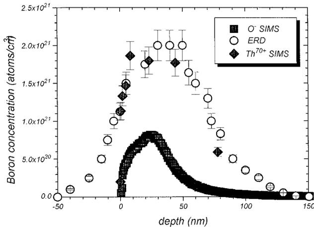
FIG. 1. Boron concentration in the B-SiO<sub>2</sub>/Si films as determined by highly charged ion based TOF-SIMS (◆), elastic recoil detection (○), and standard SIMS (■).
