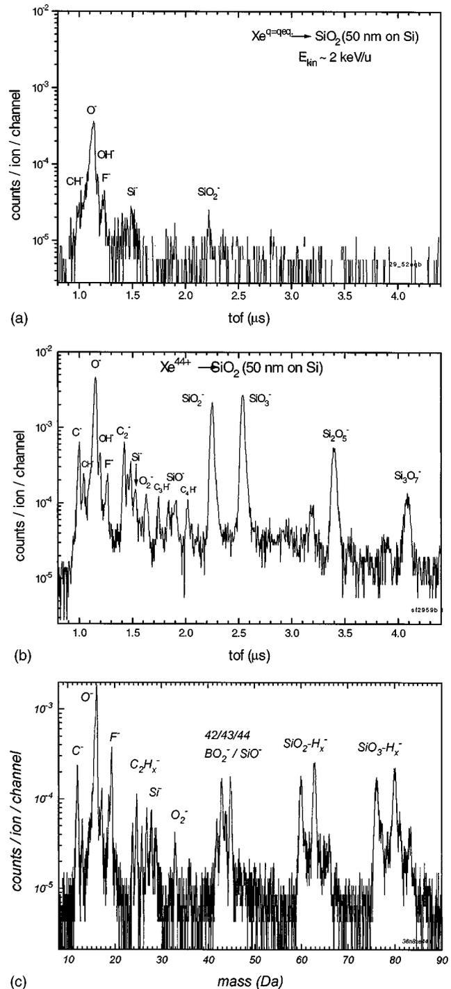
Fig. 2. Negative secondary ion spectra from thermal SiO<sub>2</sub> (50 nm on Si) at impact of xenon ions in charge state equilibrium, (a) and at impact of  $\text{Xe}^{44+}$  ions at the same kinetic energy (b). Negative secondary ion spectra from as-received 50 nm thick B-SiO<sub>2</sub>/Si films at impact of  $\text{Xe}^{44+}$  ions. The primary ion dose was  $4.6 \times 10^5$ .
